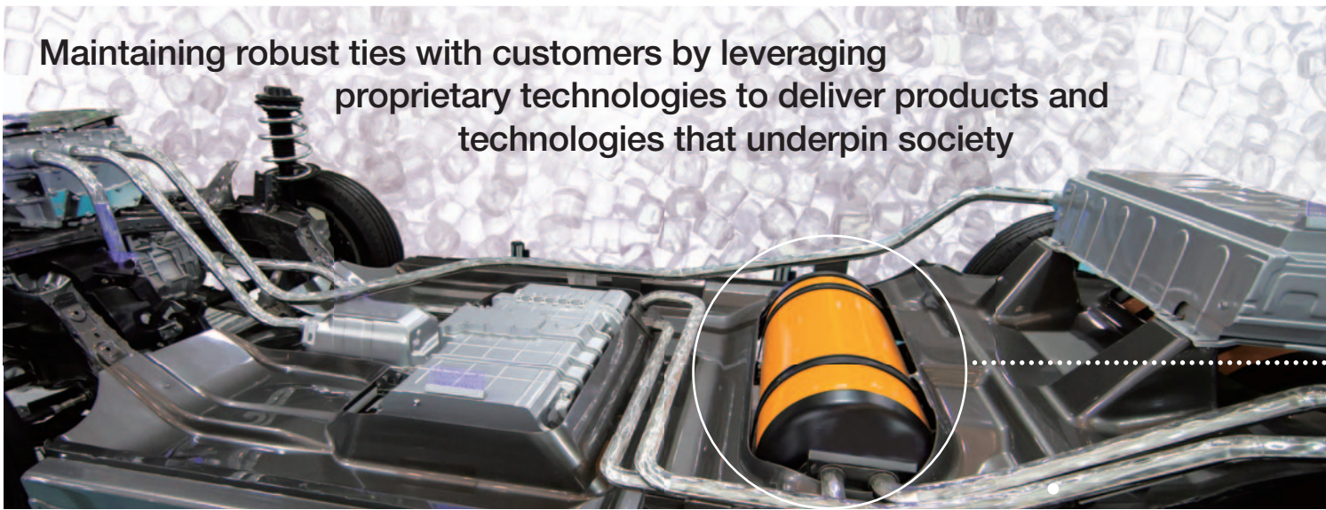
Employed in Toyota Mirai's pressurized hydrogen tank liner
