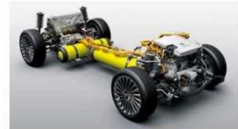
Example of nylon composite application: UBE's nylon composite used in high-pressure hydrogen tank liners for Toyota's MIRAI fuel cell vehicle. The high performance required by automotive components is achieved with engineering plastic composites.
