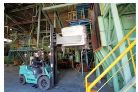
Inserting waste plastic into treatment facility
