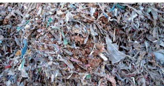
Waste plastic before treatment. Metal fragments and other foreign substances must be removed.
